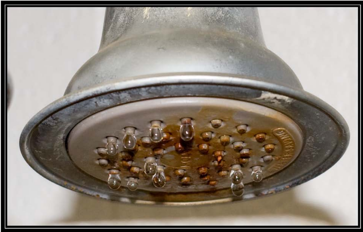
Figure 6-10C. Showerhead 10 on seventh day of testing with hard well water (28 grain per gallon) showing spray pattern. Battelle testing for Water Quality Association. May 1, 2009
