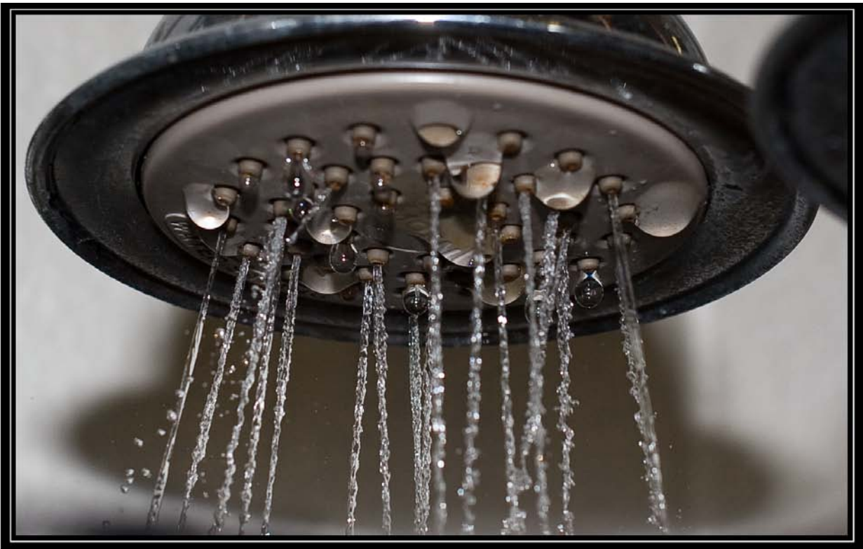
Figure 6-8B. Showerhead 8 on fourth day of testing with hard well water (25 grains per gallon) showing spray pattern. Battelle testing for Water Quality Association. April 28, 2009
