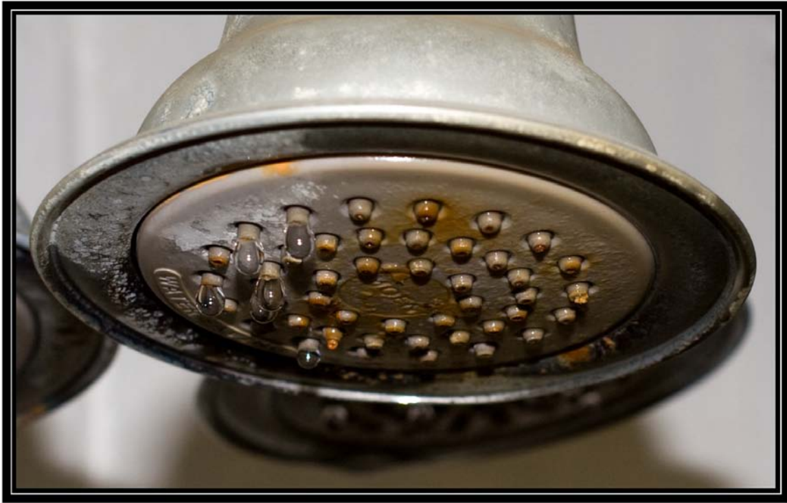
Figure 6-6C. Showerhead 6 on seventh day of testing with Hard well water (28 grains per gallon) showing condition of nozzles. Battelle testing for Water Quality Association. May 1, 2009
