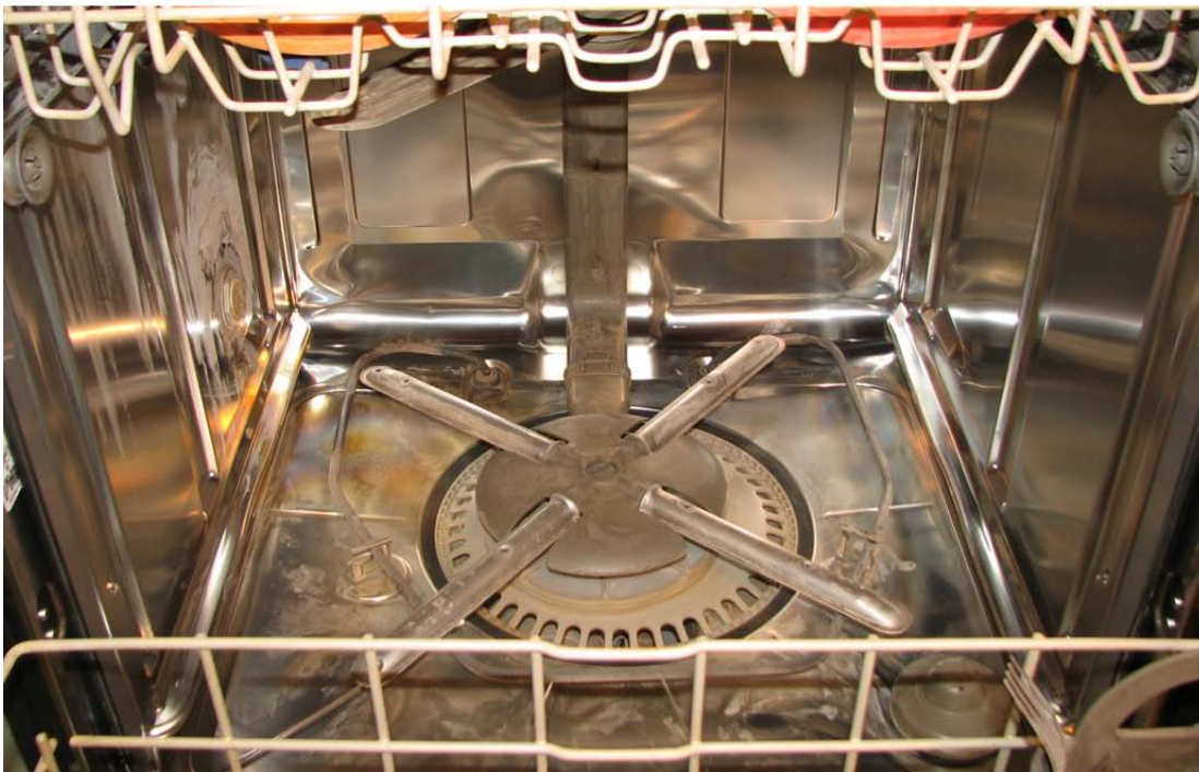
Figure 5-24. Photos showing condition of dishwasher at the end of 30 days using soft water.
