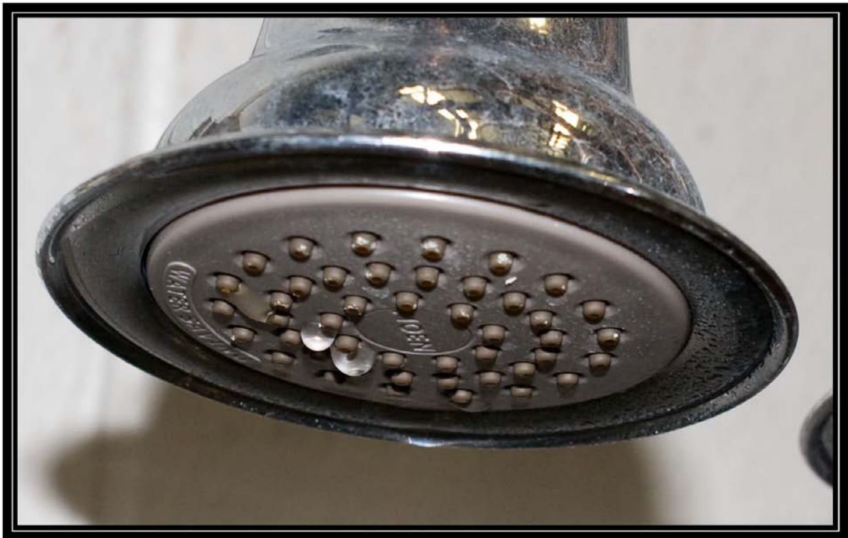
Figure 6-3C. Showerhead 3 on seventh day of testing with soft well water (<1 grain per gallon)
