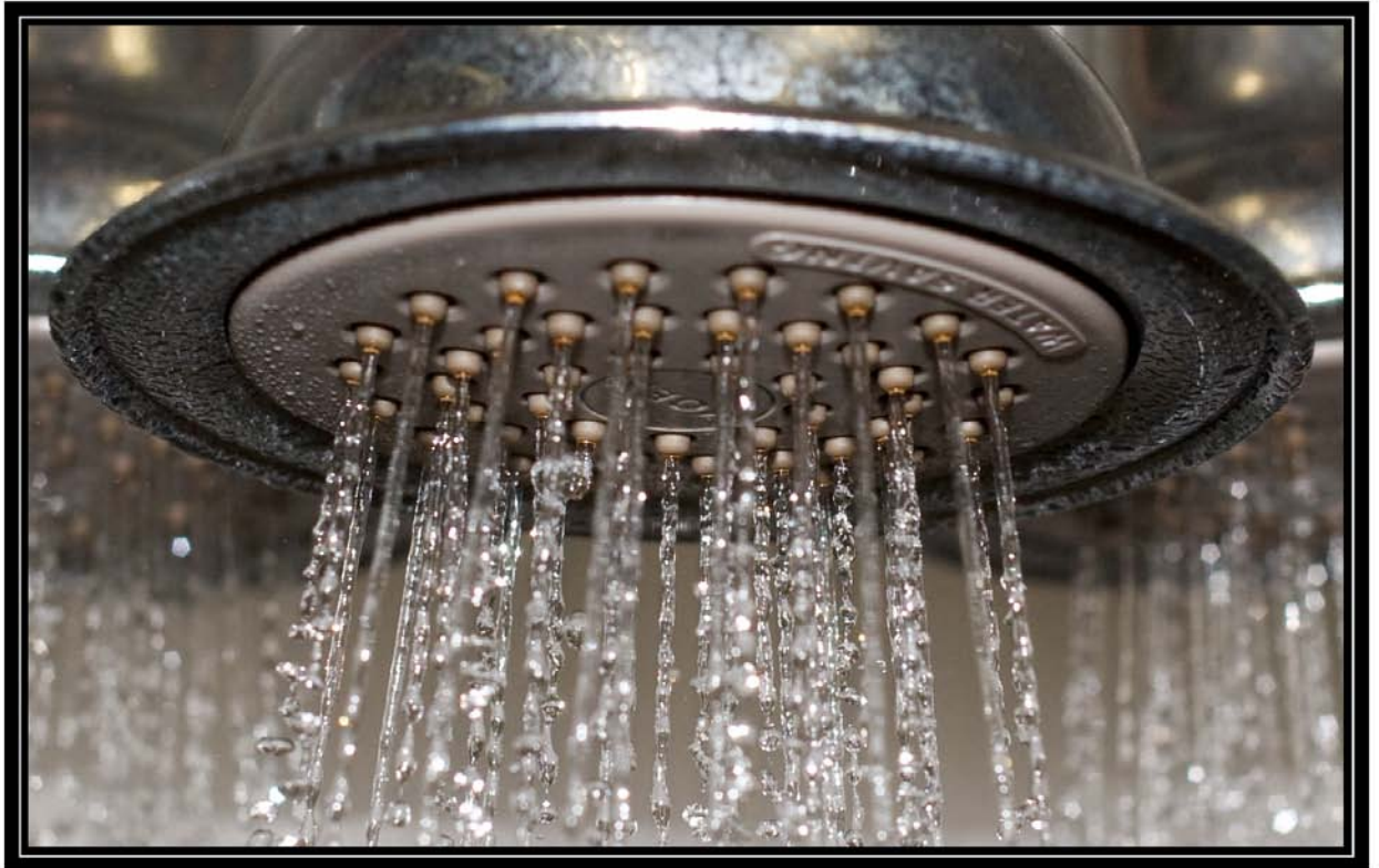
Figure 6-2D. Showerhead 2 on seventh day of testing with soft well water (<1 grain per gallon) showing spray pattern. Battelle testing for Water Quality Association. May 1, 2009
