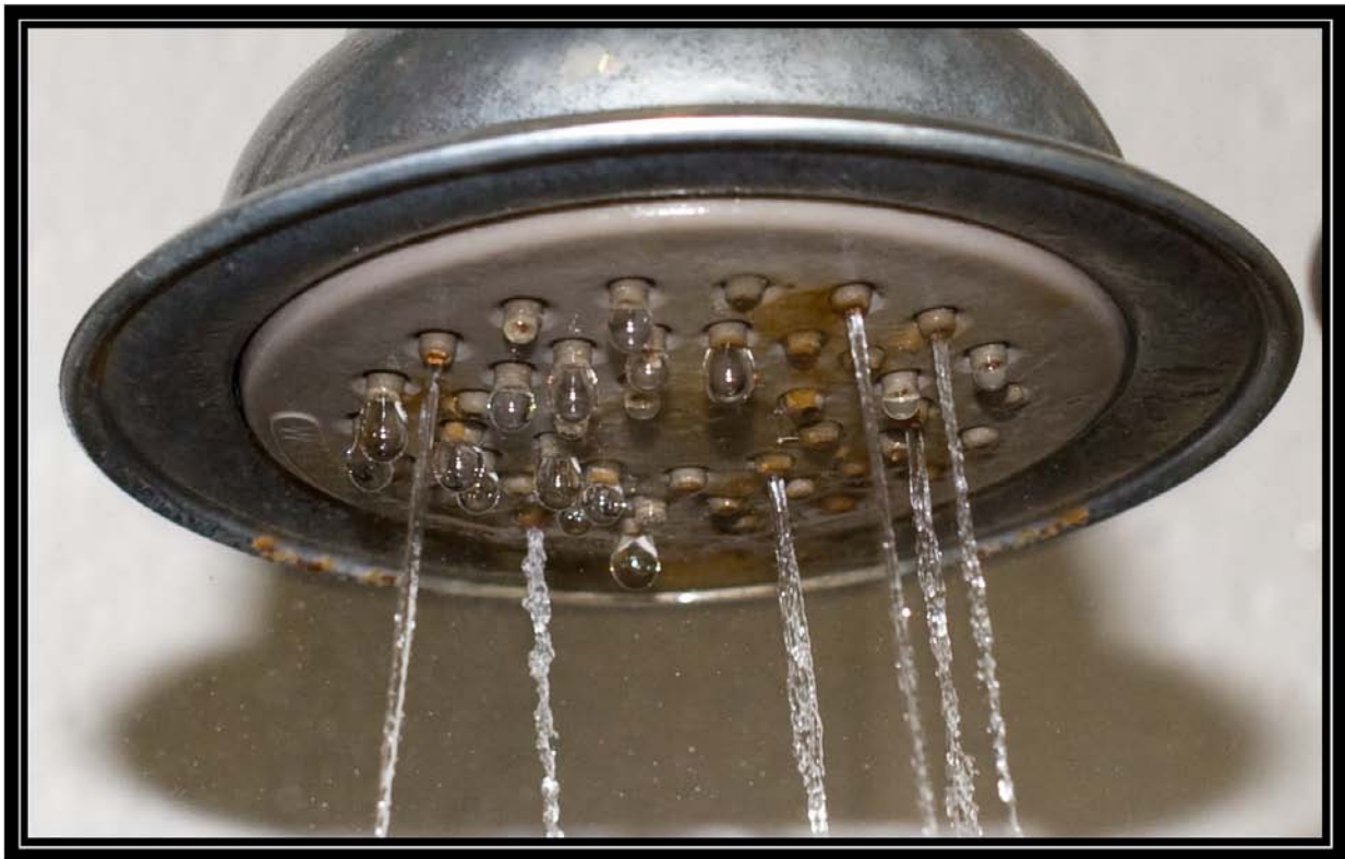
Figure 6-8D. Showerhead 8 on seventh day of testing with hard well water (28 grains per gallon) showing spray pattern. Battelle testing for Water Quality Association. May 1, 2009
