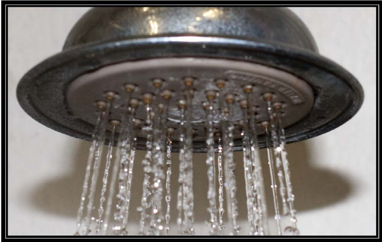
Figure 6-5D. Showerhead 5 on seventh day of testing with soft well water (<1 grain per gallon) showing spray pattern. Battelle testing for Water Quality Association. May 1, 2009
