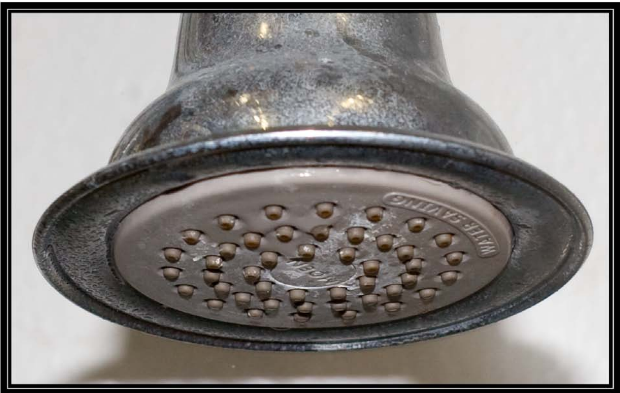
Figure 6-5C. Showerhead 5 on seventh day of testing with soft well water (<1 grain per gallon) showing condition of nozzles. Battelle testing for Water Quality Association. May 1, 2009
