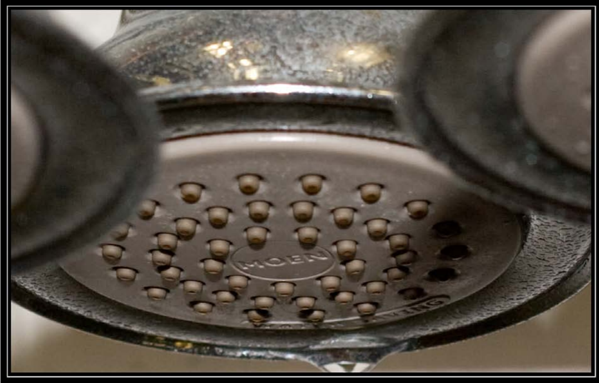
Figure 6-4C. Showerhead 4 on seventh day of testing with soft well water (<1 grain per gallon)
