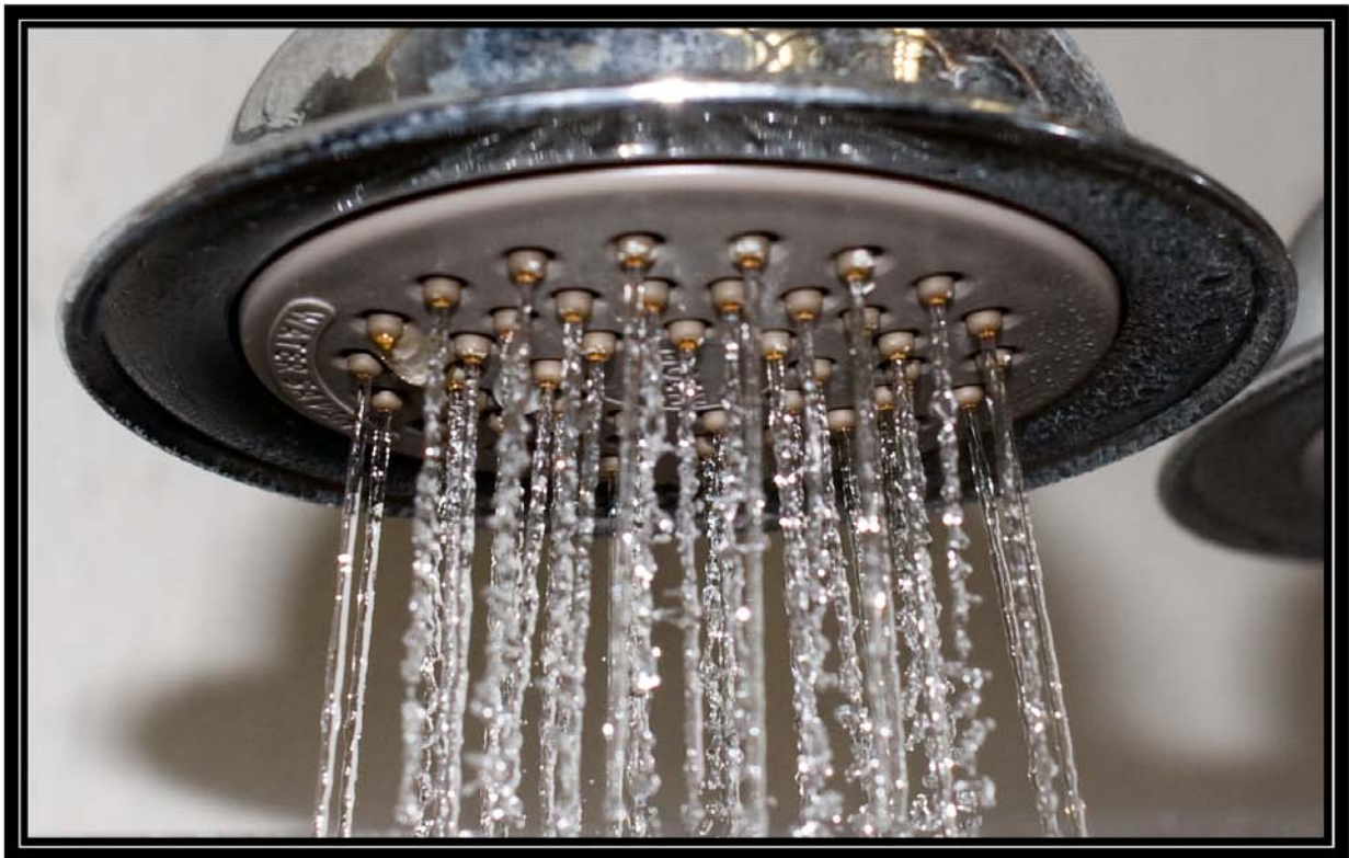
Figure 6-3D. Showerhead 3 on seventh day of testing with soft well water (<1 grain per gallon) showing spray pattern. Battelle testing for Water Quality Association. May 1, 2009
