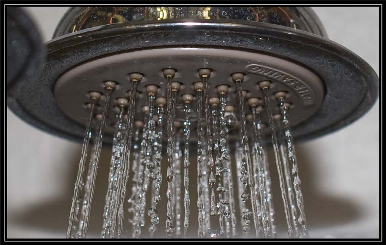
Figure 6-5B. Showerhead 5 on fourth day of testing with softened well water (<1 grains per gallon) showing spray pattern. Battelle testing for Water Quality Association. April 28, 2009
