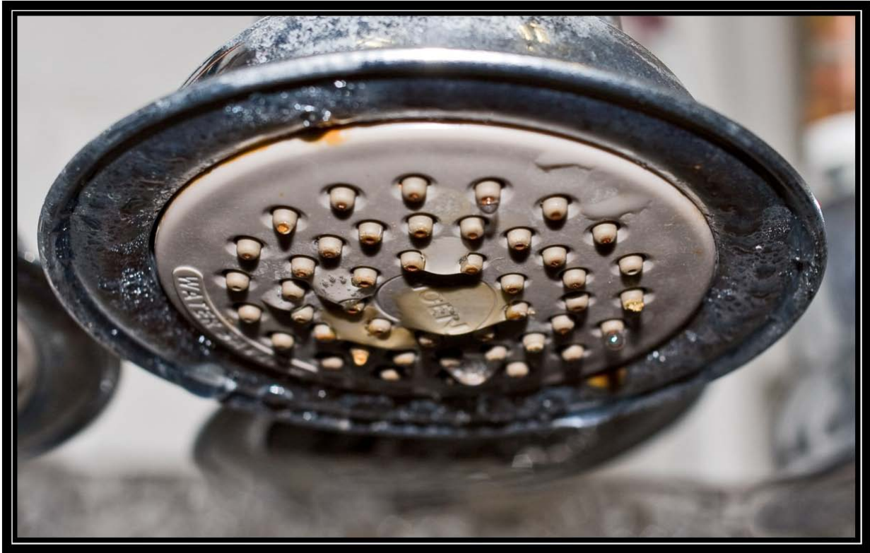
Figure 6-6A. Showerhead 6 on fourth day of testing with hard well water (25 grains per gallon) showing condition of nozzles. Battelle testing for Water Quality Association. April 28, 2009
