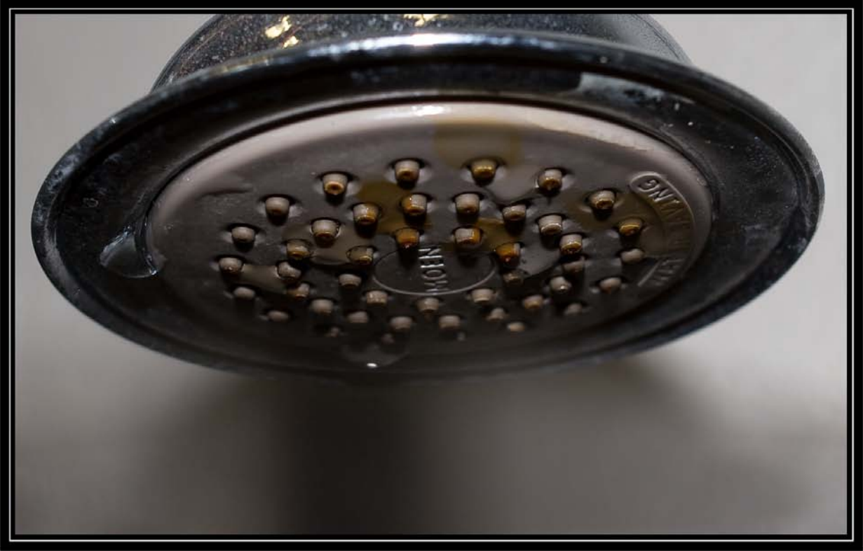
Figure 6-10A. Showerhead 10 on fourth day of testing with hard well water (25 grains per gallon) showing condition of nozzles. Battelle testing for Water Quality Association. April 28, 2009
