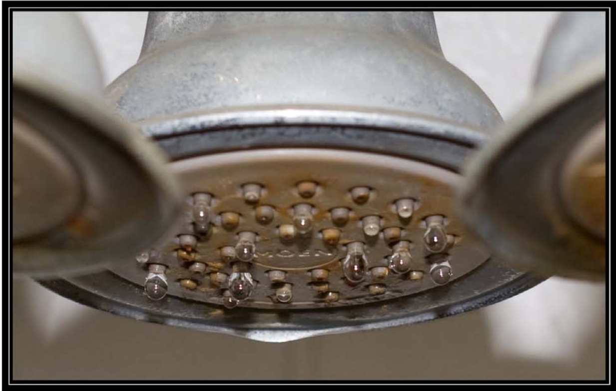
Figure 6-9C. Showerhead 9 on seventh day of testing with hard well water (28 grains per gallon) showing condition of nozzles. Battelle testing for Water Quality Association. May 1, 2009
