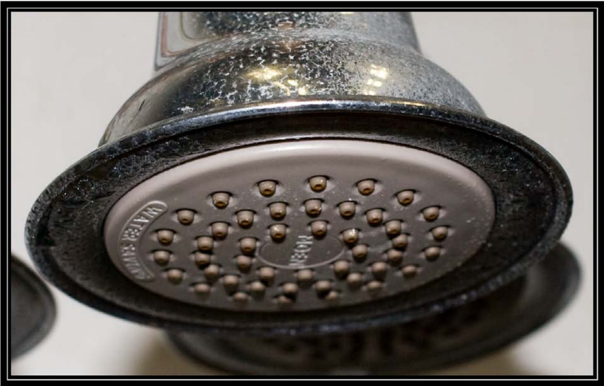
Figure 6-1C. Showerhead 1 on seventh day of testing with soft well water (<1 grain per gallon) showing condition of nozzles. Battelle testing for Water Quality Association. May 1, 2009
