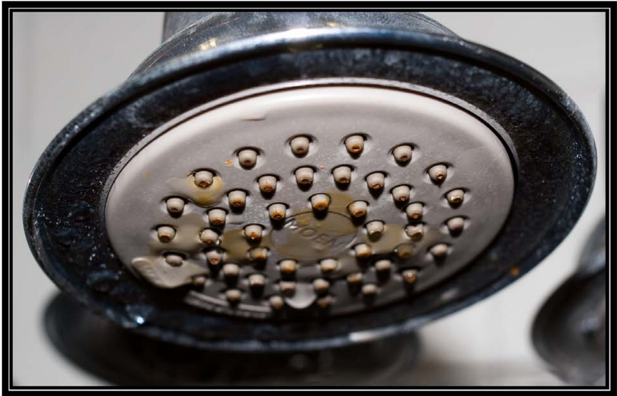
Figure 6-7A. Showerhead 7 on fourth day of testing with hard well water (25 grains per gallon) showing condition of nozzles. Battelle testing for Water Quality Association. April 28, 2009
