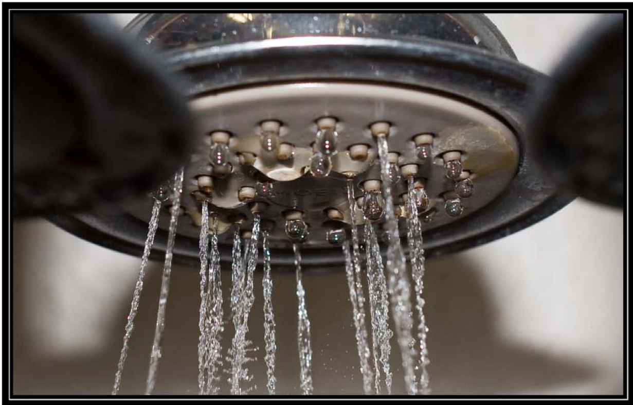
Figure 6-9B. Showerhead 9 on fourth day of testing with hard well water (25 grains per gallon) showing spray pattern. Battelle testing for Water Quality Association. April 28, 2009
