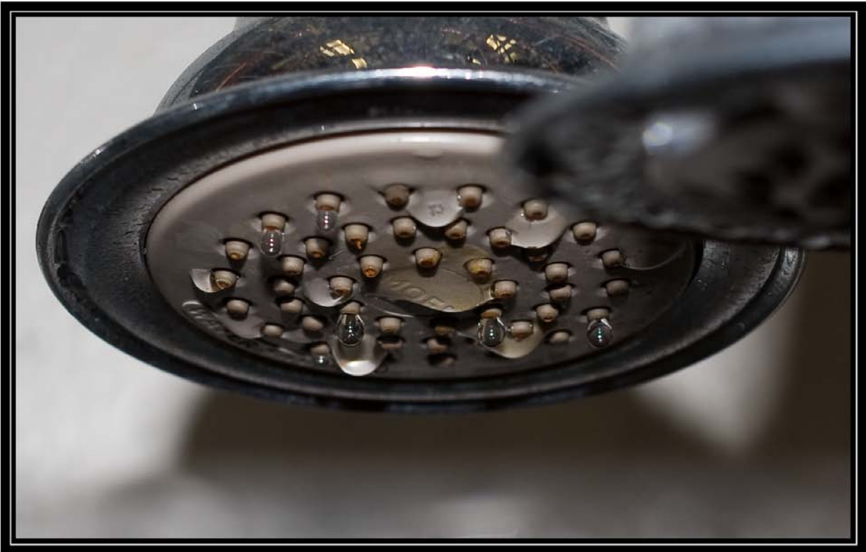
Figure 6-8A. Showerhead 8 on fourth day of testing with hard well water (25 grains per gallon) showing condition of nozzles. Battelle testing for Water Quality Association. April 28, 2009
